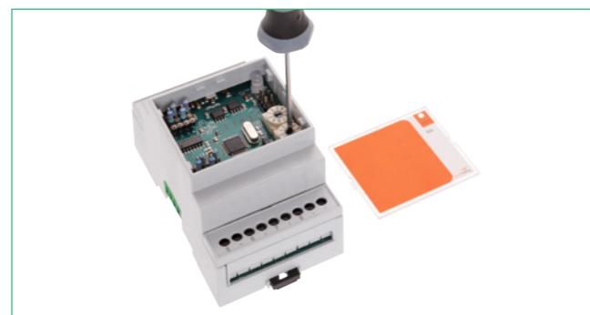
An address from 0 to 99 can be selected for the bus assignment by using the two rotary switches.
