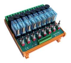
This product was designed to automatically control building blinds and lighting systems. The control system consists of relay and bypass modules that forward signals from a PLC to four groups of eight signals.
